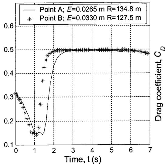
Fig. 14.  $C_D$  vs time in flight for the trajectories corresponding to both points A and B in Fig. 13. The high sensitivity of range to undercut distance can be partially attributed to the effects of the drag crisis.
