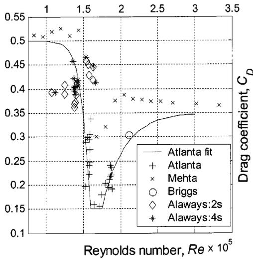
Fig. 3. Drag coefficient  $C_D$  vs Reynolds number  $Re$ . The drag decreases precipitously at  $Re\ 1.6 \times 10^5$  ( $V \sim 32\text{ m/s} = 72\text{ mph}$ ) which strongly affects the batted range.
