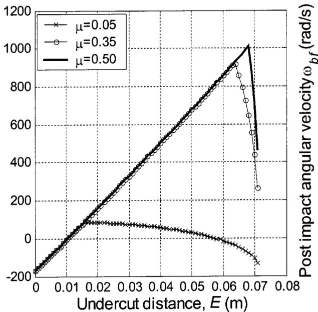
Fig. 5. Post-impact ball angular velocity  $\omega_{bf}$  vs undercut distance  $E$ . For reasonably large coefficients of friction  $0.35 < \mu < 0.5$ , the same spin is achieved for all fairly hit balls ( $\zeta < \pi/2$ ).
