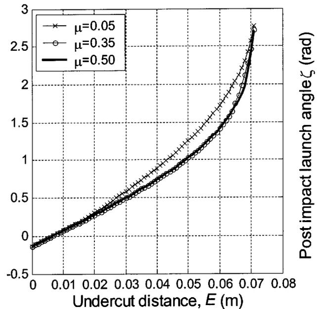
Fig. 6. Post-impact launch angle  $\zeta$  vs undercut distance  $E$ . For reasonably large coefficients of friction  $0.35 < \mu < 0.5$ , the same launch angle is achieved for all fairly hit balls ( $\zeta < \pi/2$ ).
